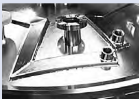
Water channel construction
