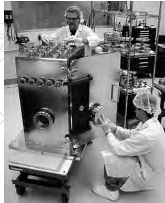
High vacuum chamber used to house an X-ray scanner in the Sandia National Laboratory LIGA project
