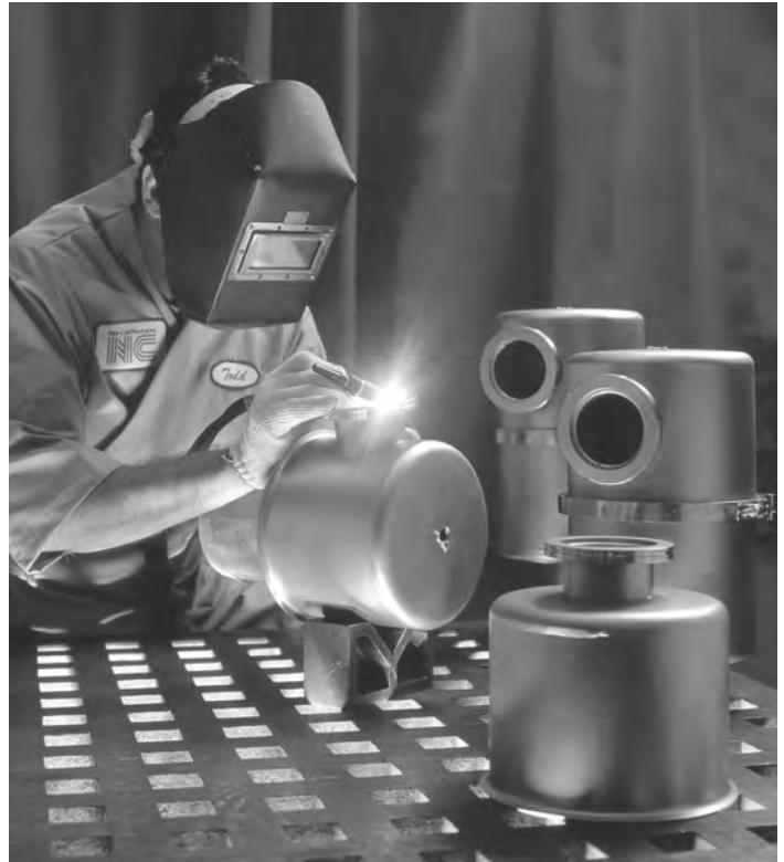
TIG Fusion Welding
