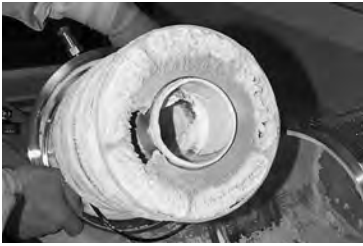
Custom water and metal sieve multistage trap
