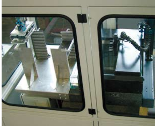
Automated Tray Scanner for analysis of IC's in JEDEC Trays
