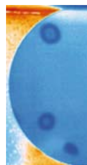
Bonded Si wafer, IR observation of the bonding interface
