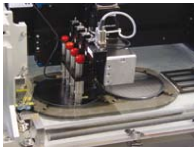
Scanning system with 4 z drives. Autofocus for each transducer
