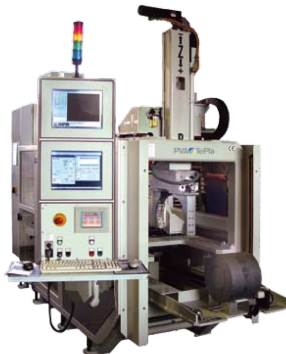
Ingot load station with gripping device
