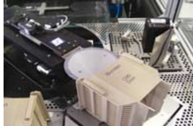
High speed robot for wafer handling
