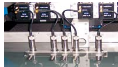
Scanner with four transducers for highest throughput of SAM investigations (T1, 2, 3, 4)
