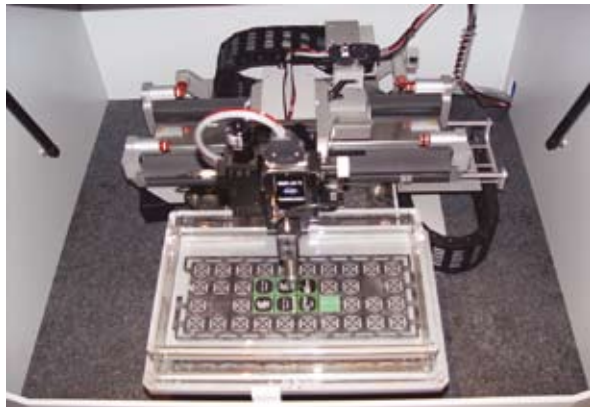
Air support linear motion scanner for high throughput acoustic analysis, maintenance free
