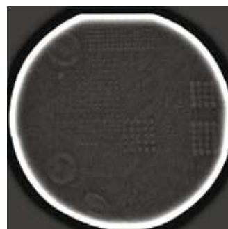
Bonded Si wafer, X-ray observation of the bonding interface
